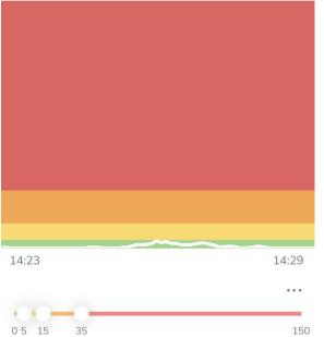
In Scenario 5, the background concentration was  $1\mu g/m^3$  prior to idling with a relatively short but steady increase to a peak of  $5\mu g/m^3$ , some oscillation during the idling of 2-3 minutes, and a quick decrease to background levels, when the idling stopped.
