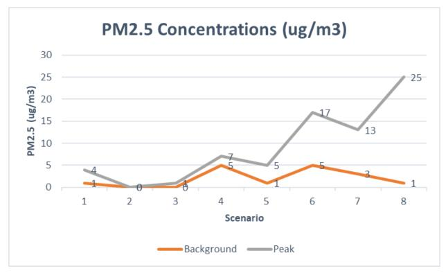
The graph above shows the background and peak concentrations of PM2.5 (vertical axis) recorded inside the vehicle in all eight scenarios (numbered 1-8 on the horizontal axis) of the experiment.
